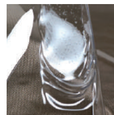
A clear visor molten by radiant heat
