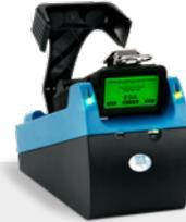
The GfG test stations offer fast, automatic and cost-effective execution of daily bump tests including documentation according to DGUV information 213-056 (T021) and 213-057 (T023). In addition, the docking stations also enable the required, routine functional checks to be carried out.
